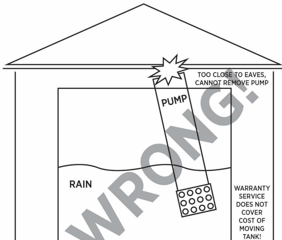
NO APPLIANCE LASTS FOREVER. INSTALLATION MUST ALLOW FOR REMOVAL FOR SERVICING OR REPAIRS.
