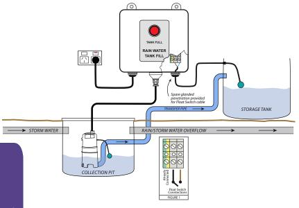
This simple, yet effective controller provides the means of controlling an automatic pump, used to transfer stormwater from a collection pit to a storage tank. This system has low voltage supply to the float switch, situated in the storage tank, and the controller. When the storage tank is full, the controller isolates the pump and the 'tank full' light is illuminated. An IP68 connector is provided for a waterproof connection for the float switch cable at the storage tank.
