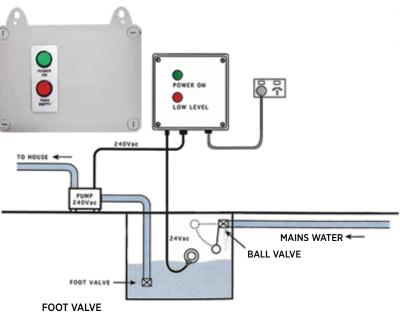
This simple, yet effective controller provides the means of controlling an automatic pump, used to pump water from a tank into the home. The system uses low voltage between the float switch, situated in the storage tank, and the controller. When the storage tank is empty, the controller isolates the pump and the 'Low Level' light is illuminated. Power to the pump is restored once water level in the tank has risen to the reset level.
