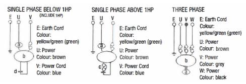
THREE PHASE PUMPS must be connected to a external motor starter fitted with a contactor and overload. The nominal current of the motor starter must correspond to the electrical data marked on the pump nameplate.
