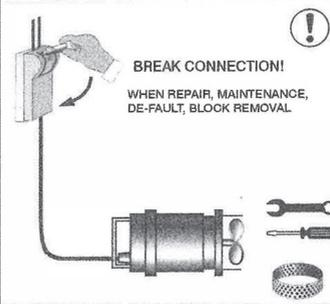
BREAK CONNECTION! WHEN REPAIR, MAINTENANCE, DE-FAULT, BLOCK REMOVAL
