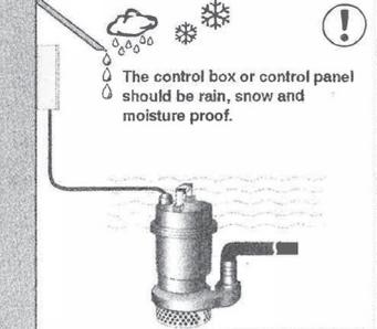
The control box or control panel should be rain, snow and moisture proof.
