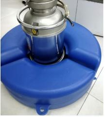
3. Attach suitable rope to the float ring through the loops provided, for the purpose of positioning the pump, and also to enable retrieval if ever necessary.
