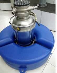
2. Place the pump in the centre of the float ring, and ensure that the 3 brackets holding the support ring on the pump slot into the join between each float segment.
