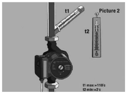
Max Water Temp: 100°C Max Ambient Temp: 40°C Min Water Temp: 5°C Min Ambient Temp: 2°C
