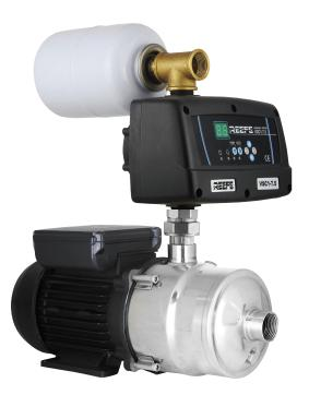
\*The SP value can be set to the desired output pressure irrespective of the incoming mains pressure. However, this value MUST NOT exceed the sum of the Incoming Mains pressure value plus (80% of the rated pressure of the pump). Be mindful, too, of the 500kPA limitation on household fittings.
