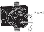
The regulated pressure should be at least 1 bar less than the maximum pressure of the pump.
